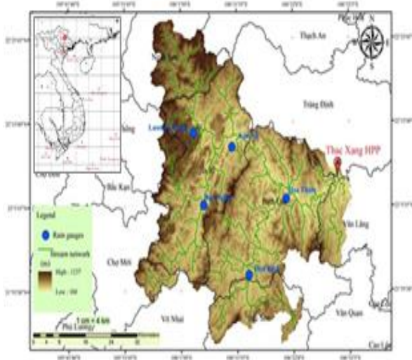
Figure 5. Thac Xang reservoir drainage basin and stream network.
